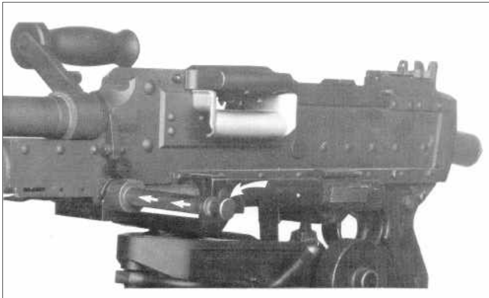
Figure 4-9 Inserting the Front Mounting Pin
