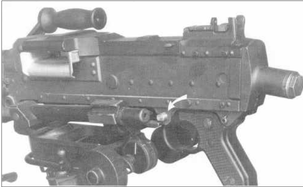
Figure 4-8 Correct Position of the Rear Mounting Pin
